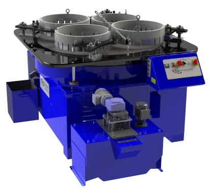
The Lapmaster Wolters model 56 is equipped with a 1422mm diameter lap plate. This is manufactured from Grade 300 grey cast iron to ISO 185(2005). It consists of individual segments bolted to a support plate.
